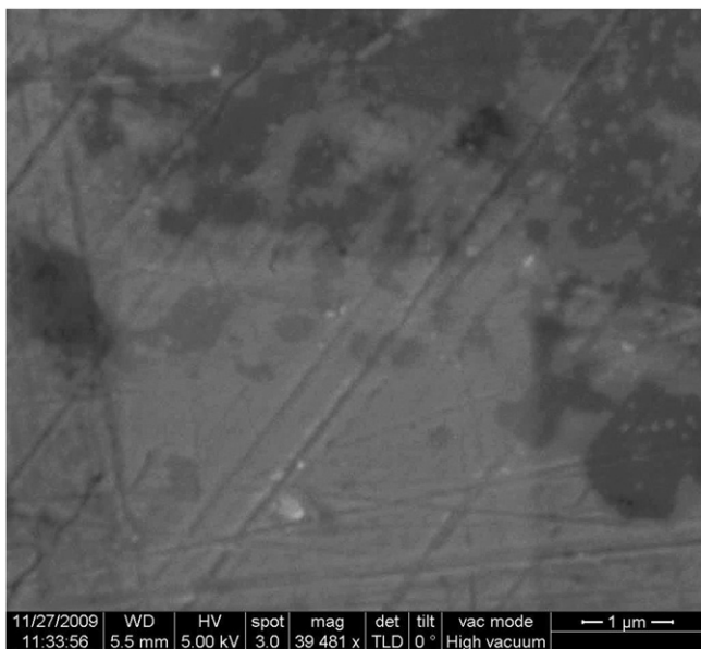
Fig. 3. High resolution SEM showing features of a few 100 nm on sample \text{Pb}_{0.55}\text{Sn}_{0.10}\text{Ge}_{0.35}\text{Te} .
